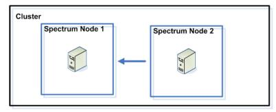
As you add additional nodes, the new nodes can point to any of the existing nodes as a seed node. You must also configure the first node to point to at least one other node in the cluster so that if it is ever brought down it can rejoin the cluster.
