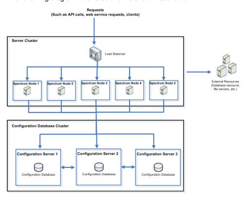
To install a separate database repository, you first install the configuration database on servers in a cluster, then install the server on nodes in a separate cluster. At least one configuration database must be running before you can install the server.
