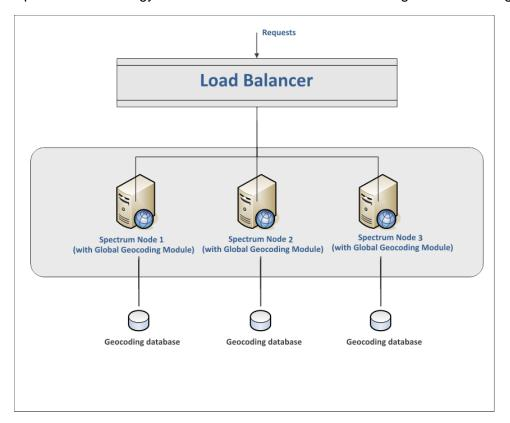
**Note:** Each Geocoding database MUST be installed in the same location on all of the nodes for the cluster to work properly. For example, if the Geocoding database for "Spectrum Node 1" is installed on C:\data\, then the other Spectrum nodes' Geocoding database must also reside on C:\data\.
